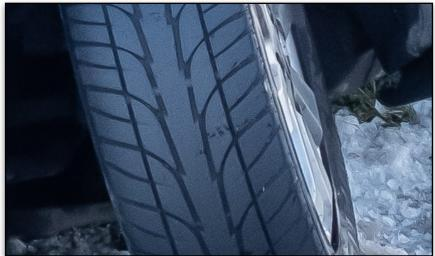
In this case the nearside front tyre is worn down to the tread wear indicators ie no more than 1.6mm.
