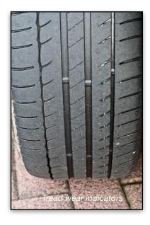
The deeper the tread the more water the tyre can disperse and the greater your grip on the road. Look for the tread-wear indicators on your tyres (see picture) - if they are flush with the tread the tyres need replacing.
